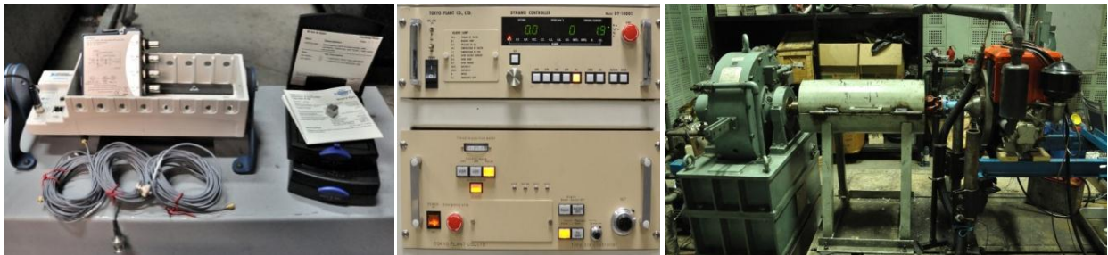
Fig. 4 An experimental set up for vibration load measurement: (from left) DAQ equipments and accelerometer, dynamometer load controller, and dynamometer chassis with test engine.
